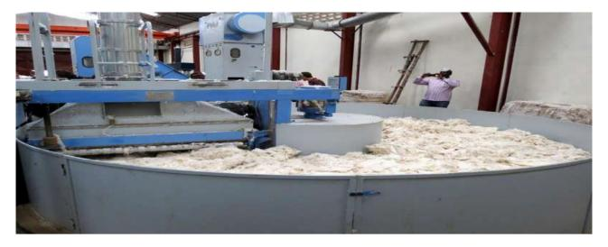
The lint cotton received from the ginning machine is sent for further cleaning. This process involves cleaning of the impurities; therefore it runs through cleaning equipment to remove leaf trash, sticks and other foreign matter.
